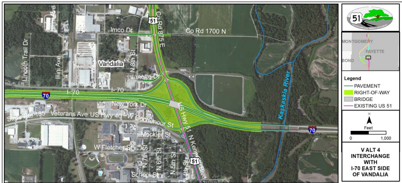
Figure 2.3-19: V Alt 4 Reconfiguration of Existing Interchange with I-70 on the East Side of Vandalia
