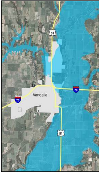
The Kaskaskia River floodplain is extensive on the east and south sides of Vandalia. The regulatory floodplain is shown in blue.
